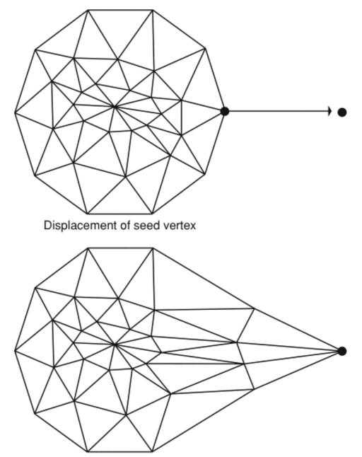
Attenuated displacement propagated to adjacent vertices
