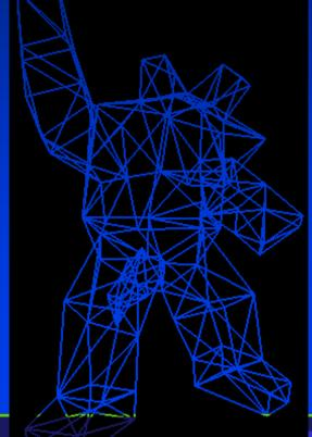
• Low-resolution auxiliary shape controls deformation of high-resolution model
