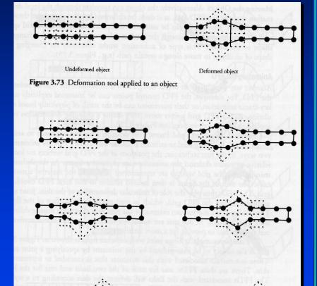
Figure 3.74 Deformation by translating the deformation tool relative to an object
