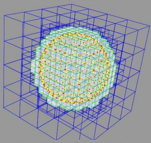
Octree containing pieces of an implicitly defined sphere; within each terminal node surface vertices are computed and connected to form a polygon
