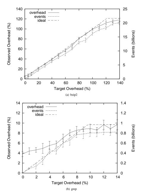
Fig. 16. Cascade controller with range-solver observed overhead (y-axis) for a range of target overhead settings (x-axis) and two workloads.
