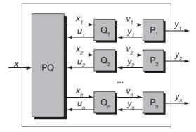
Fig. 6. Overall cascade control architecture.
