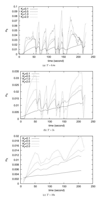
Fig. 21. Local target monitoring percentage  $(m_{lt})$  over time during bzip2 workload for range-solver with cascade control. Results shown with target overhead set to 20% for 4 different values of  $K_I$  and 3 values of T.
