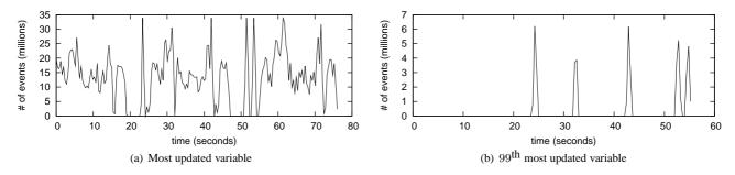
**Fig. 14.** Event distribution histogram for the most updated variable (a) and  $99^{th}$  most updated variable (b) in bzip2. Execution time (x-axis) is split into 0.4 second buckets. The y-axis shows the number of events in each time bucket.
