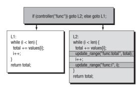
Fig. 11. range-solver adds a distributor with a call to the SMCO controller. The distributed passes control to either the original, uninstrumented function body shown on the left, or the instrumented copy shown on the right.
