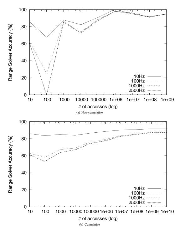
Fig. 20. Accuracy of global controller clock frequencies with 4 different clock frequencies using range-solver instrumentation. Variables are grouped by total number of updates.
