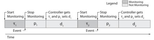
Fig. 8. Timeline for secondary controller.
