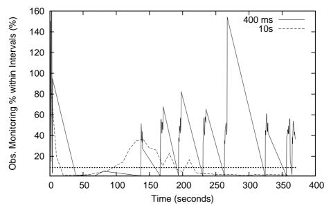
Fig. 24. Observed monitoring percentage over bzip2 range-solver execution. The percent of each adjustment interval spent monitoring for 2 values of T. The target monitoring percentage is shown as a dotted horizontal line.
