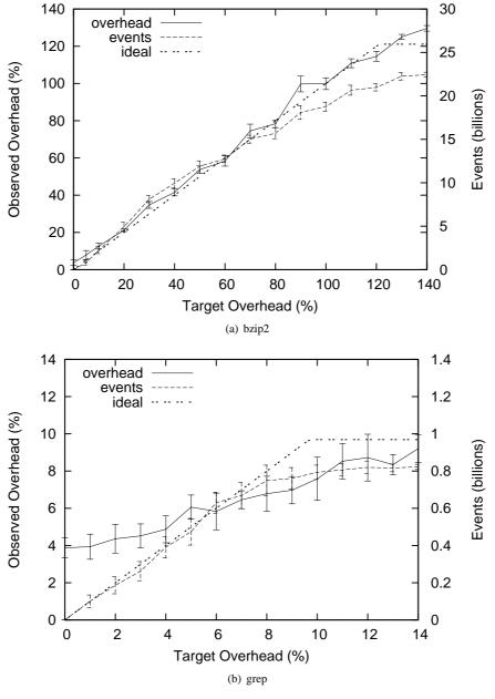
Fig. 15. Global controller with range-solver observed overhead (y-axis) for a range of target overhead settings (x-axis) and two workloads.
