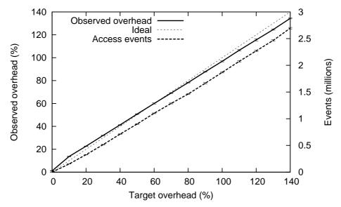
Fig. 18. Cascade controller with NAP detector observed overhead (y-axis) and number of monitored memory access events (y2-axis) for a range of target overhead settings (x-axis) running on the bzip2 workload.
