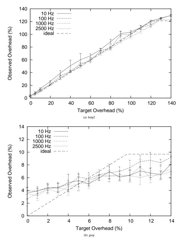
Fig. 19. Observed overhead for global controller clock frequencies with 4 different clock frequencies and 2 workloads using range-solver instrumentation.
