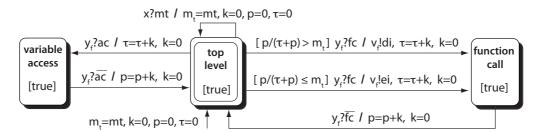
Fig. 5. Automaton for global controller.
