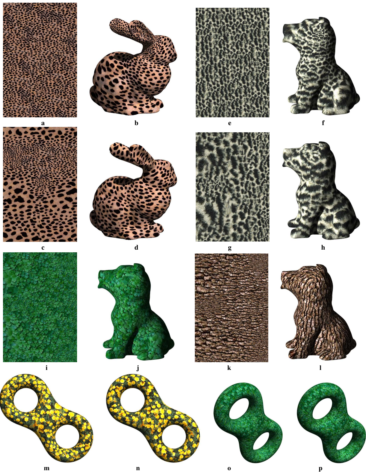
Fig. 9 Multi-scale texture synthesis results. (a),(e) uniform texture synthesized on geometry images without considering area stretching factor; (b),(f) nonuniform texture by mapping (a) and (e) onto 3D surfaces; (c),(g) nonuniform texture synthesis considering area stretching factor; (d),(h) uniform texture by mapping (c) and (g) onto 3D surfaces; (i)-(l) more uniform texture synthesis results; (m),(o) nonuniform textures on 3D surfaces, texture features inside the handles are smaller than those outside; (n),(p) uniform textures on 3D surfaces. High resolution images as well as videos can be obtained at http://www.cs.sunysb.edu/~lujin/paper/pg05/ .
