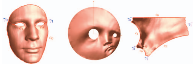
Fig. 6. A triply connected domain can be conformally mapped onto a planar disk with two circular holes using euclidean Ricci flow, and the fingerprint (conformal module) is the centers and radii of the inner circular holes. It can also be mapped onto the Poincaré disk periodically using hyperbolic Ricci flow, with all boundaries becoming geodesics. The lengths of the boundaries are the conformal module.
