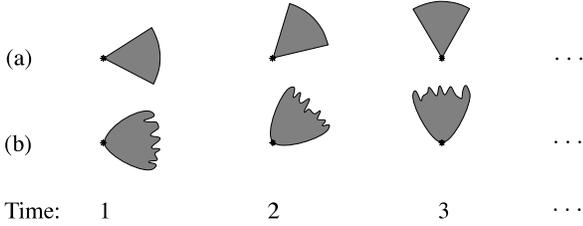
Fig. 1. Examples of *rotating directional sensors* with (a) cone-shaped sensing regions, and (b) more general sensing regions. The initial orientation (time slot 1) is towards right. The RDS rotate anti-clockwise.
