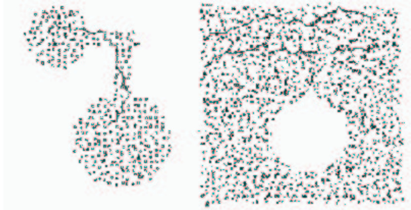
Figure 5: Examples of routes generated by GLIDER. L: Narrow corridor connecting 2 rooms, R: Dense network with small and large holes
