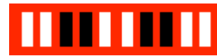
Figure 2. Red code for the number 9 (1001). The left half mirrors the right half of the code.
