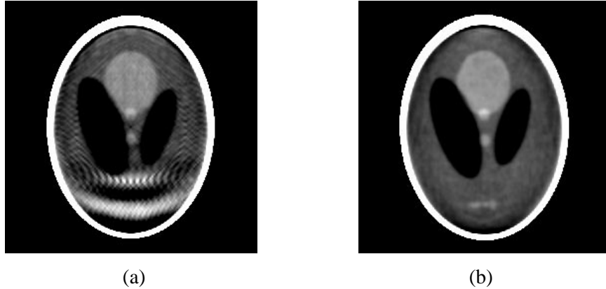
Fig. 2. (a) The slice of Fig. 1a reconstructed with traditional ART from cone-beam projection data ( \lambda=0.08 , \gamma=60^\circ , \mathbf{V}^{(0)}=\mathbf{0} , 3 iterations, 80 projections). Notice the significant stripe artifacts that completely obliterate the small tumors. (b) A reconstruction of the same slice from parallel beam data using the same algorithm and parameter settings. This reconstruction does not have the strong artifacts of (a).
