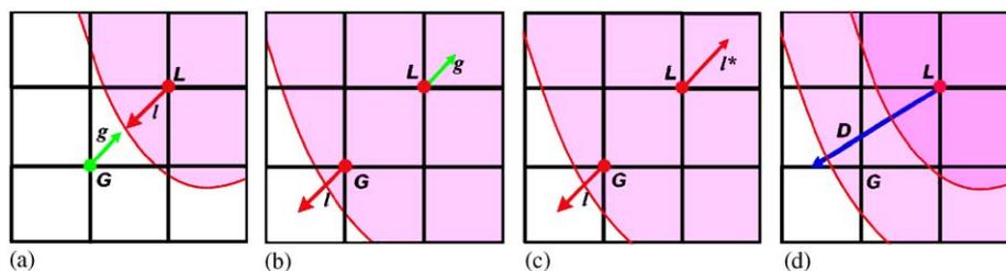
Fig. 3. Liquid (pink) and gas (white) interface. (a) Particle distributions between gas cell  $G$  and liquid cell  $L$ ; (b) unmodified streaming results: gas particles flow into liquid improperly; (c) modified streaming results: gas particles are replaced by liquid particles; (d) liquid mass is dragged forward by a body force  $D$ .
