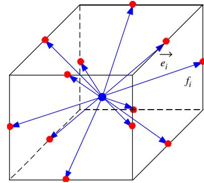
Fig. 1. The D3Q13 lattice geometry. The particle distribution  $f_i$  is associated with the link corresponding to the  $\mathbf{e}_i$  velocity vector from a lattice site (blue) to its neighbors (red).
