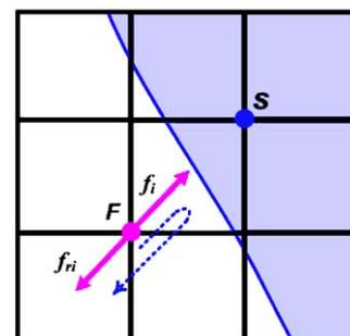
Fig. 2. Bounce back rule for solid–fluid interface.
