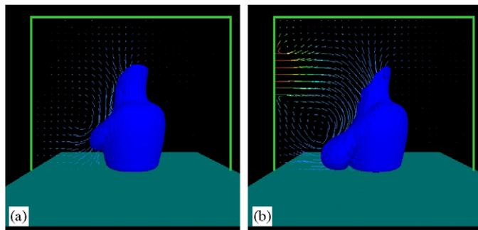
Fig. 5. Velocity field streamlines of a melting vase. (a) No wind; (b) with wind from the heat source.
