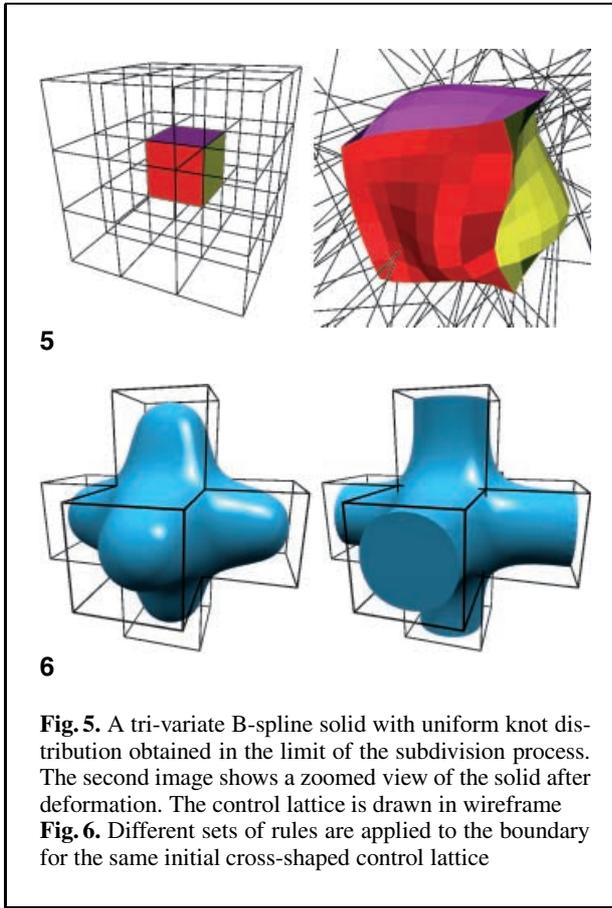
**Fig. 5.** A tri-variate B-spline solid with uniform knot distribution obtained in the limit of the subdivision process. The second image shows a zoomed view of the solid after deformation. The control lattice is drawn in wireframe
