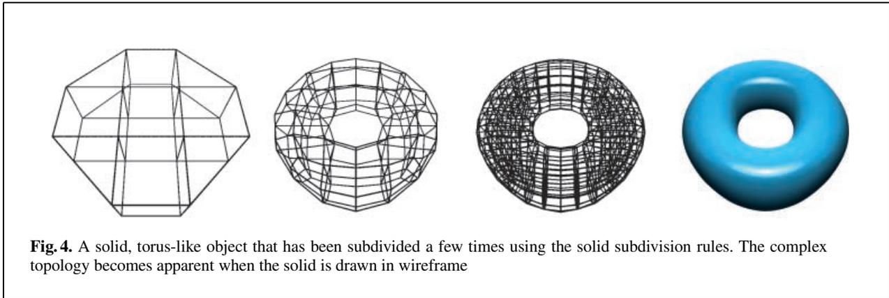
ric MacCracken–Joy subdivision scheme as a novel free-form spline solid that is obtained in the limit through recursive application of subdivision rules on a user-specified lattice of control vertices.
