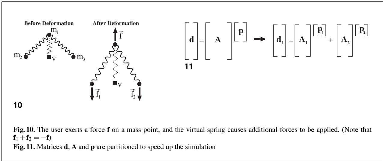
oscillations and to bring the system to an eventual rest state. We then divide the force acting on each point by the mass in order to compute the point's acceleration. The positions of the virtual points are updated. Finally, we compute the accelerations of the control points using Eq. (10) and update their positions. At any time during the simulation, the user may modify the object's topology, and the system will rebuild the necessary data structures to effect the change.
