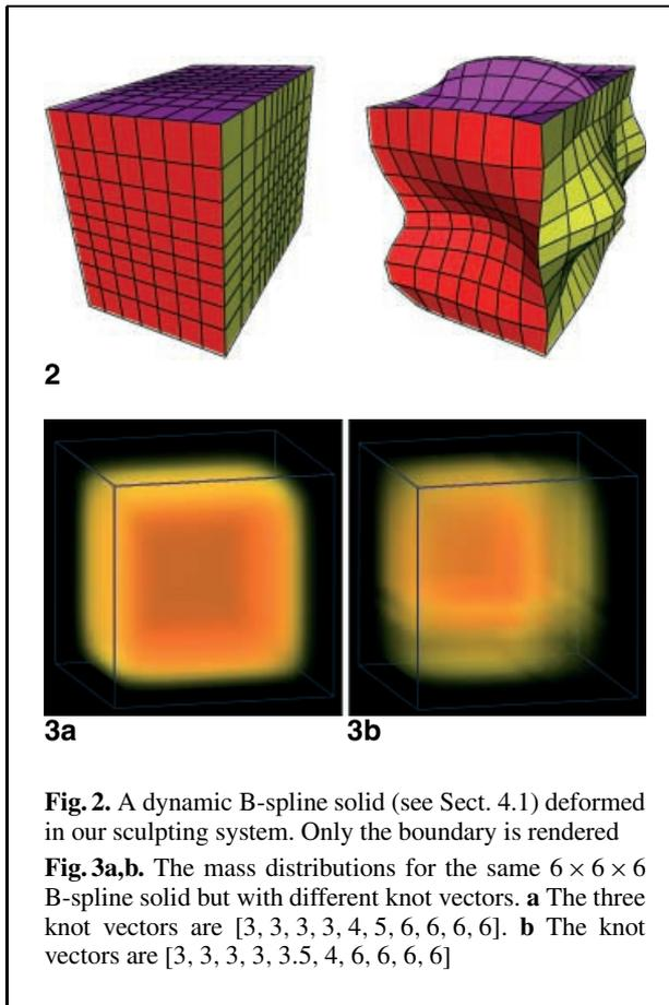
**Fig. 2.** A dynamic B-spline solid (see Sect. 4.1) deformed in our sculpting system. Only the boundary is rendered
