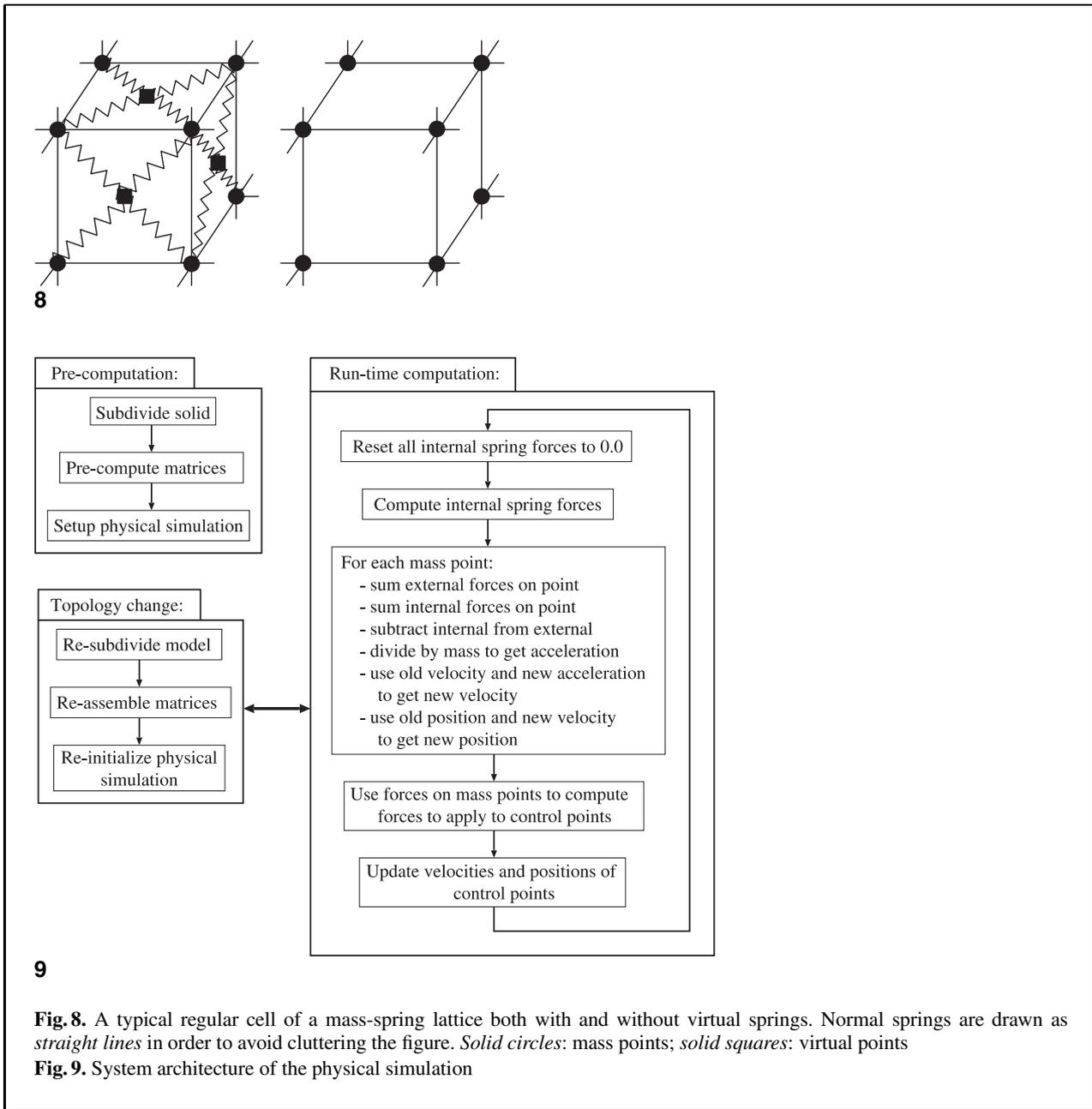
ing the simulation, the system evolves as follows: First, all internal forces are reset to zero. Second, for each spring, the force exerted on each mass point attached to the spring is computed by Hooke's law:  $\mathbf{f} = -k(\mathbf{l} - \mathbf{l}_0)$ , where  $\mathbf{l}_0$  is the spring's rest length. Third, the forces exerted by the virtual springs are taken into account, again using Hooke's law. After we compute the force exerted on the mass point that
