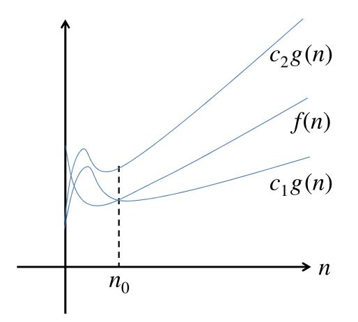
$\Theta(g(n)) = \begin{cases} f(n): \text{there exist positive constants } c_1, c_2 \text{ and } n_0 \text{ such that} \\ 0 \le c_1 g(n) \le f(n) \le c_2 g(n) \text{ for all } n \ge n_0 \end{cases}$
