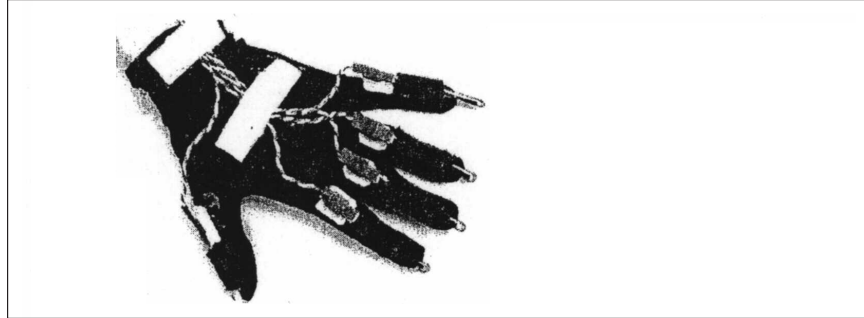
Figure 2. Our data glove for capturing hand signs. It is designed mostly from off the shelf parts. Touch sensors are embedded inside the globe, while the bend sensors are on the outside.
